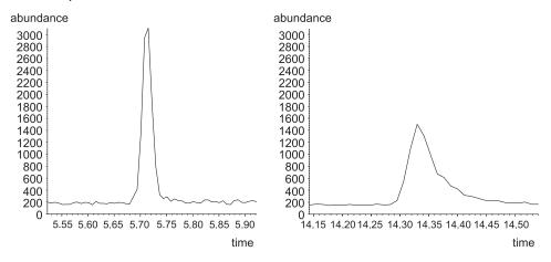
Fig. 1. Peak-shapes of chlorothalonil obtained by LP-GC/MS and GC/MS
