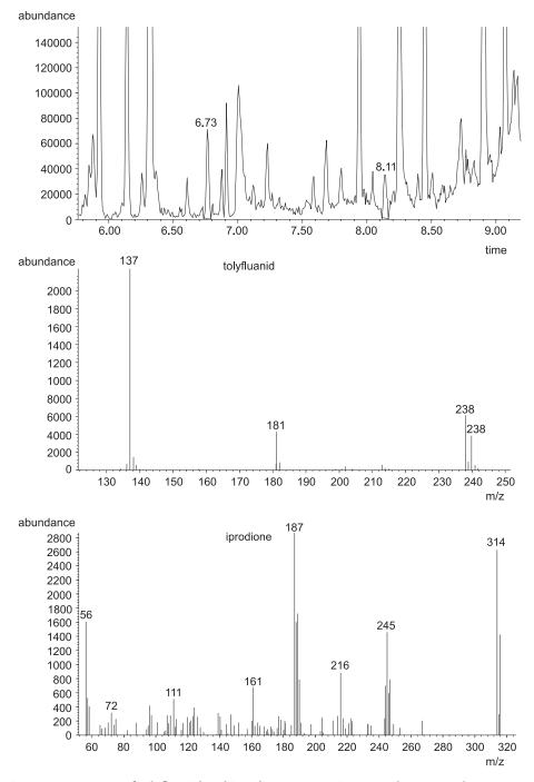
Fig. 2. Mass spectra of tolyfluanid and iprodione present in a strawberry sample
